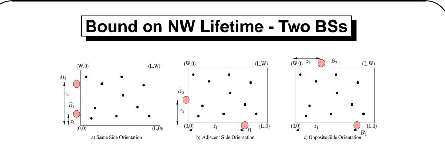
**Figure5:** *Placements of two base stations. a) Same side orientation, b) adjacent side orientation, and c) opposite side orientation*
