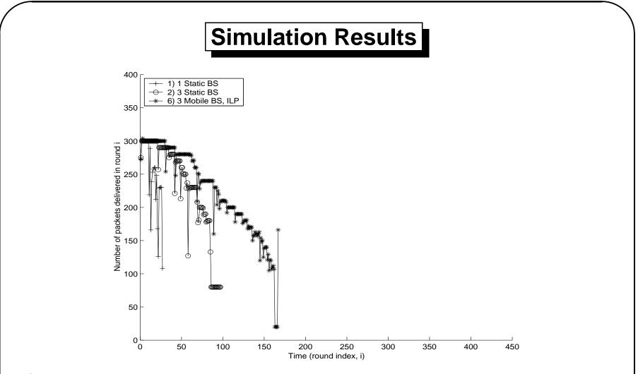
**Figure 11:** Traces of number of packets delivered per round as a function of time for schemes 1), 2), and 6). MCF routing. Initial energy at each node,  $E_{battery} = 0.05$  J. One packet = 200 bits. Range of each node, r = 10 m.
