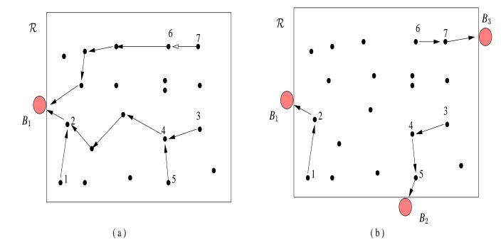
**Figure1:** A sensor network over a rectangular region of observation  $\mathcal{R}$  with three base stations  $B_1, B_2, B_3$ . Node 1 sends its data to base station  $B_1$  via node 2. Node 3 sends its data to  $B_2$  via nodes 4 and 5. Node 6 sends its data to  $B_3$  via node 7. However in Single base station case data has to travel more no. of hops.
