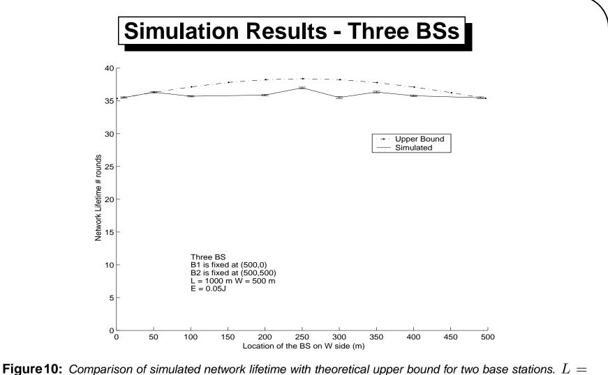
**Figure 10:** Comparison of simulated network lifetime with theoretical upper bound for two base stations.  $L = 1000 \text{ m}, W = 500, E_{\text{battery}} = 0.05 \text{ J}. B_1$  fixed at (500,0).  $B_2$  fixed at (500, 500). Location of  $B_3$  varied from (0,0) to (0,500)
