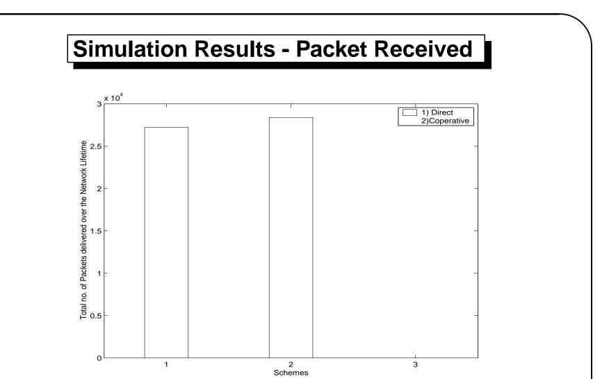
**Figure 20:** Comparison of the no. of Packets Received for Direct and Cooperative case over the duration of Lifetime.  $L = 1000 \text{ m}, W = 500 \text{ m}, E_{\text{battery}} = 0.5 \text{ J}.$
