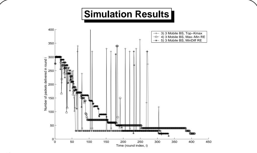
**Figure 12:** Traces of number of packets delivered per round as a function of time for the proposed schemes 3), 4), and 5). MCF routing. Initial energy at each node,  $E_{battery} = 0.05$  J. One packet = 200 bits. Range of each node, r = 10 m.
