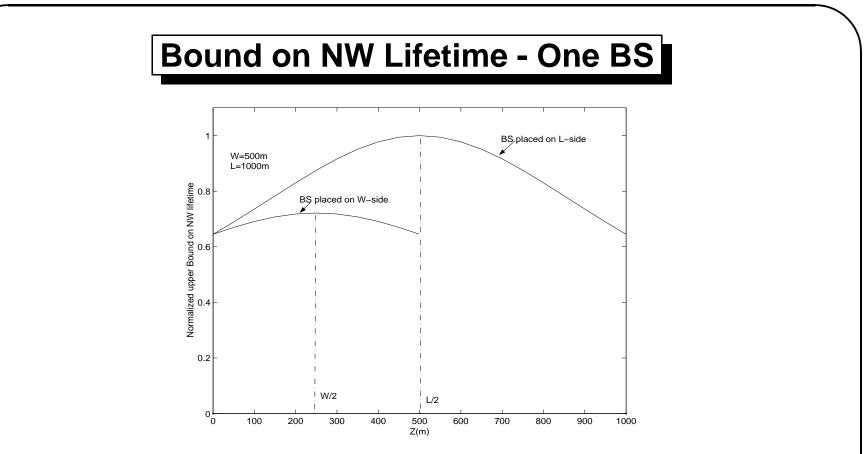
**Figure4:** Normalized upper bound on network life time as a function of base station location for L = 1000 mand W = 500 m
